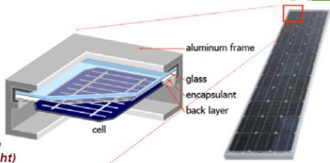
**Single PV cell (left) and constructive details of a photovoltaic module (right)**
