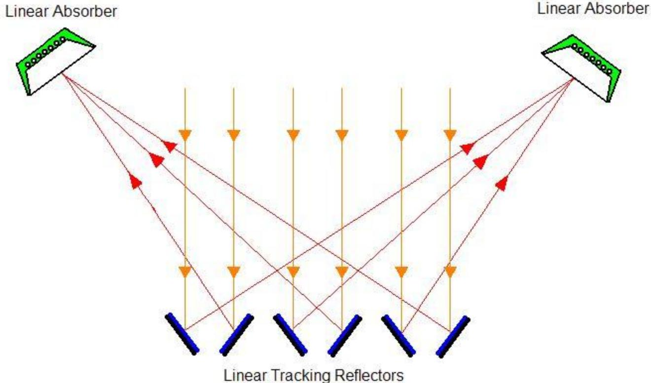
CLFR solar systems alternate the inclination of their mirrors to focus solar energy on multiple absorbers, improving system efficiency and reducing overall cost. The concept also reduce the foot print by about 30% compared to LFR
