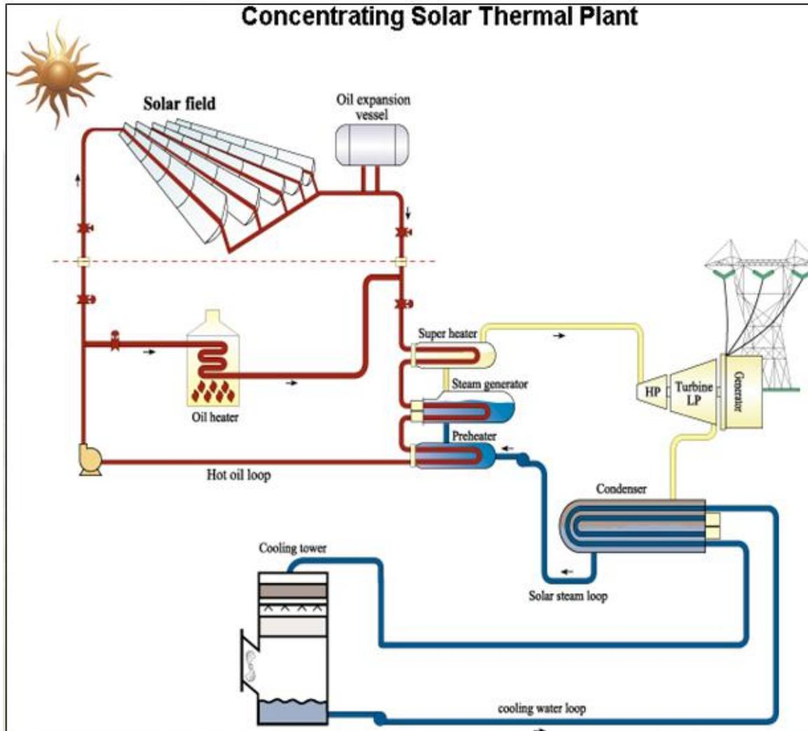
Schematic diagram of a solar-thermal energy conversion system.
